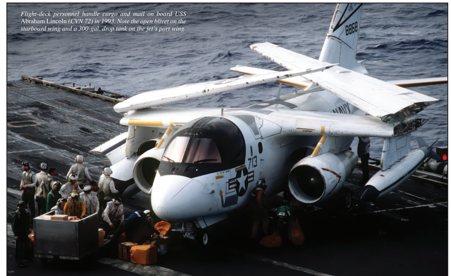
A close-up of “Miss Piggy” surrounded by mail representing the most valued service of the Viking COD. The artwork was positioned between the normal crew window and the added slit window, which was the only external difference between the S-3 and US-3.
