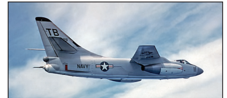
A3D-1, BuNo 135429, pictured in flight. Note the defensive tail armament that was part of the airplane's original specifications. VAH-1's “TB” tailcode honored CAPT Tom Blackburn, the HATWING-1 commander and World War II fighter ace while skipper of the famed VF-17 Jolly Rogers.
