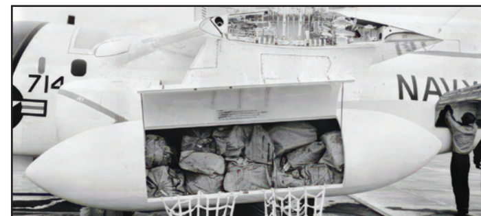
A fully packed blivet with cargo restraining nets pictured on the port wing of a US-3A. The blivet measured 18 feet, 8 inches and weighed 460 pounds before being packed with cargo.
